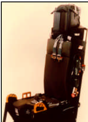
ACES II seat, all systems self-contained, pilots merely strap in
